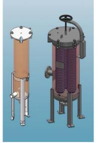
CUNO offers the HC Series housings, for use with 3M 700 Series Filter Cartridges in 1, 3, 5 and 7 around housing configurations. Constructed with 304L or 316L stainless steel, the housings are designed for use with 28 <sup>3</sup>/<sub>4</sub>" and 39" length filter cartridges. The housings are rated for operation up to 10 bar @ 90°C and manufactured in accordance to design and construction code EN13445 Group 3.
