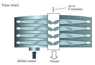
The frame structure of the module is made of polypropylene. A stable, metal-free core sleeve carries the drainage body, which supports the filter sheets. The defied medium is forced under pressure through the filter material. The sediment particles are retained and the filtrate is passed through the drainage body, and the core sleeve to the outlet. The seal between the modules and to the filter housing is either a flat adaptor or a bayonet adaptor with double O-ring.
